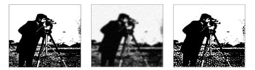
FIGURE 13. Deblurring and denoising: original image (left), damaged image with blur and noise effects (middle), reconstructed image for  $\alpha = 2.10^{-4} \sqrt{n}$  (right).
