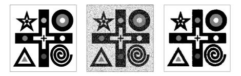
FIGURE 6. Greylevel image denoising with update of levels (3 labels),  $L^1$  norm,  $\alpha = 5.10^{-3}\sqrt{n}$ : original image (left), noisy image (middle) solution with 3 labels (right) and  $\alpha = 5.10^{-3}$ .
